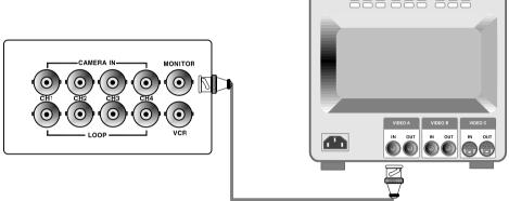
Connect the video output MONITOR to Video-In of Main monitor.
